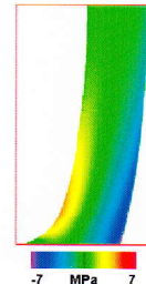
Axial stress distribution in the wall in three sections
